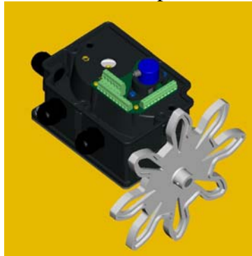
Picture 6 –Rendering of the PCB board and mini incremental encoder
